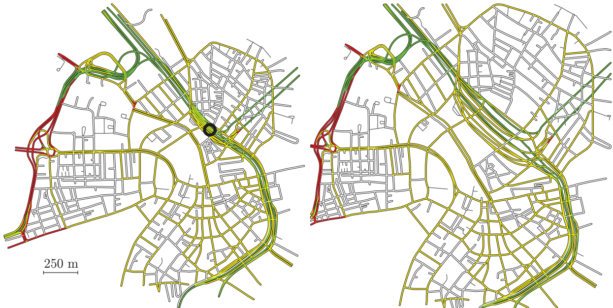
Fig. 1. A road map of Boston (left). A user selects a focus region (black circle) and sets a zoom factor Z , here Z = 3 . Then, an output map (right) is generated. The focus region is scaled up by Z while the map still fits into its original frame. This is achieved by scaling some parts of the road network down that are not in the focus region. Distortions at road segments of the network are minimized.
