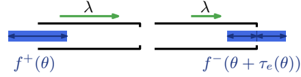
Fig. 3. An illustration of how the flow rate changes depending on the speed limits. On the left: As the speed limit \lambda is high, the flow volume entering the arc per time unit is represented by the area of the long rectangle. On the right: The speed limit is halved, and therefore, the same amount of flow needs twice as much time to leave the arc (or enter the queue if there is one). Hence, if there is no queue, the outflow rate at time \tau + \tau_e(\theta) is only half the size of the inflow rate at time \theta .
